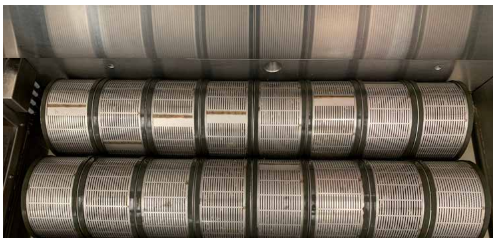
GRL photo collection: cages with barley grain during malting in the Phoenix micromalting unit
