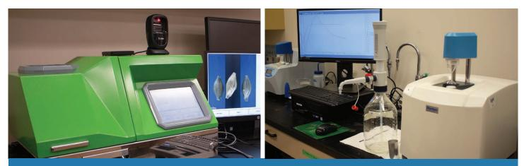
Cgrain Value image analyzer (left) and Rapid Visco Analyzer (right) used by the barley program at the Grain Research Laboratory.
